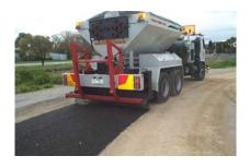
2.4m width of spray sealing, easily selected control with 300mm segments or narrow strips.
