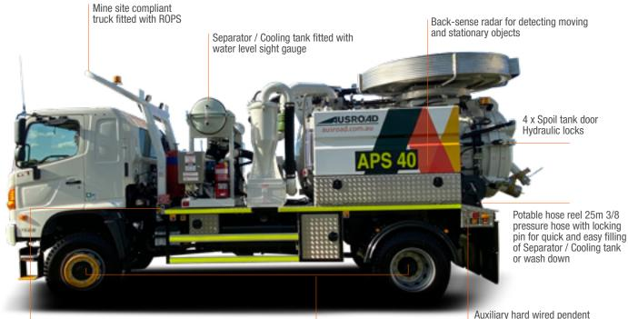
The latest cutting edge in earthing system. Earth-rite static earthing system does not allow Vac section to work if no earth is found or lost during excavation
