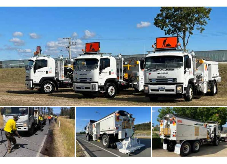
Designed to deliver asphalt or quarry products and is suitable for a variety of road maintenance requirements.
