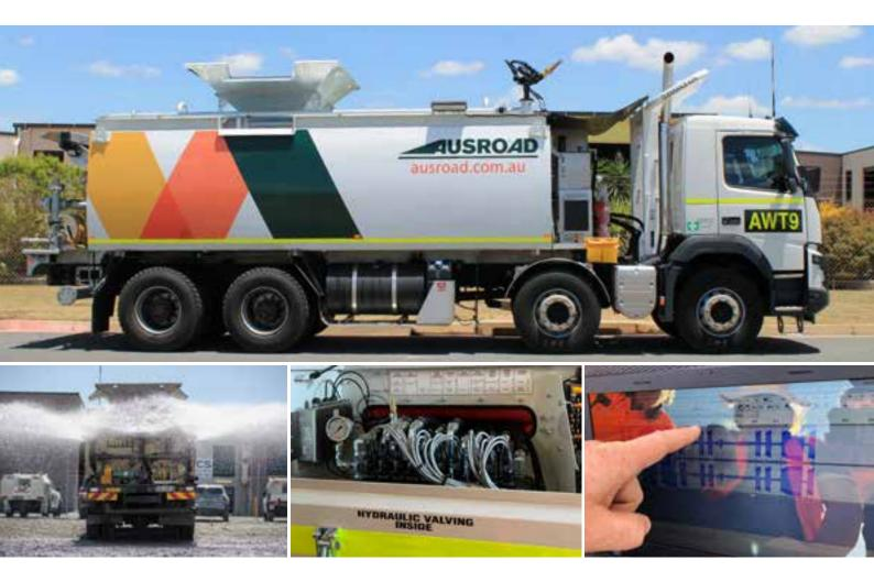
Most processes are fully controlled from the driver's seat, enhancing safety, proportional hydraulic control allows accurate control of pump speed.
