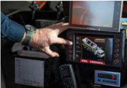
• State of the art control system. Reverse camera, load cell system with transmission lock out, automated calibrated delivery, blast design software integration
