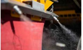
• Dust suppression on discharge of material to protect ground crew
