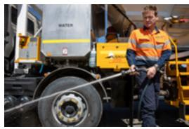
• Wash down hose with hydraulic pump and 3000L water tank
