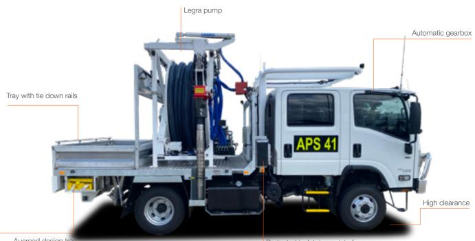
Ausroad design tray built to handle the mines
