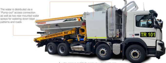
A water cannon and high-pressure water pump can be fitted to aid wash down of equipment.
