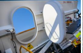
• Hydraulic operated hopper hatch
