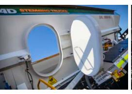
Hydraulic operated hopper hatch
