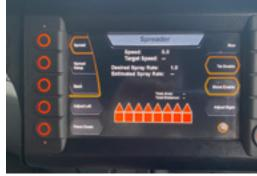
Operator interface is set out in a logical layout to provide effortless function control with remote access support options.
