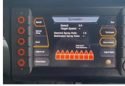
• Operator interface is set out in a logical layout to provide effortless function control with remote access support options.
