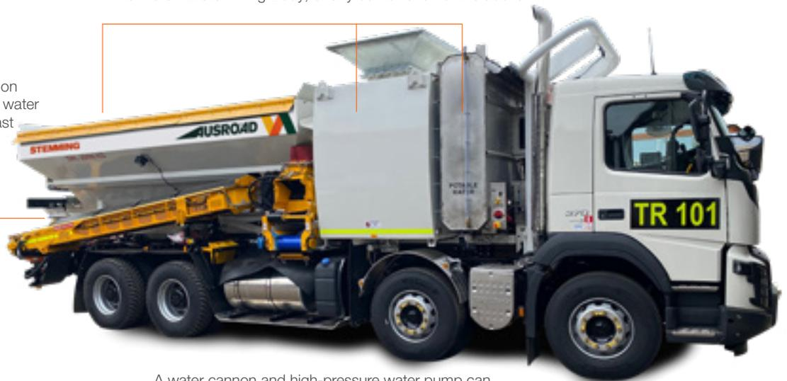
A water cannon and high-pressure water pump can be fitted to aid wash down of equipment.
