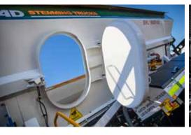
Hydraulic operated hopper hatch
