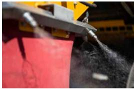
Dust suppression on discharge of material to protect ground crew
