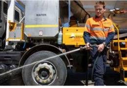
Wash down hose with hydraulic pump and 3000L water tank
